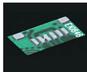
桥连 Short circuit
