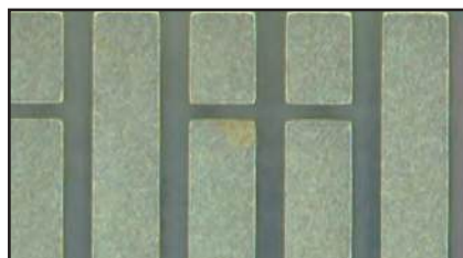
金面污染 Gold surface contamination
